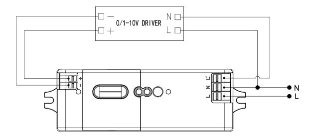
\*The sensor is designed for connect one load only. Connect more than one loads may damage the sensor.
